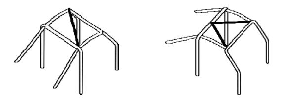
Tube which runs longitudinal from one of the highest points of the B-bar to the other side of the Abar, must also be reinforced in each corner according to the drawing beside. A space of minimum five cm between helmet and tubes is recommended.
